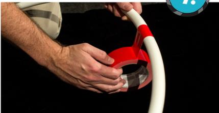
Cover the connection all the way around with electrical tape or duct tape. This fastens your tube into a hoop shape.
